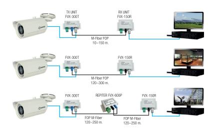
They solve all the problems associated with conventional video cables: distance of the video signal, poor image quality and "jerky images" due to the RF noises, difficulty in laying the cable in undersized ducts, coexistence with other cables, etc ...
